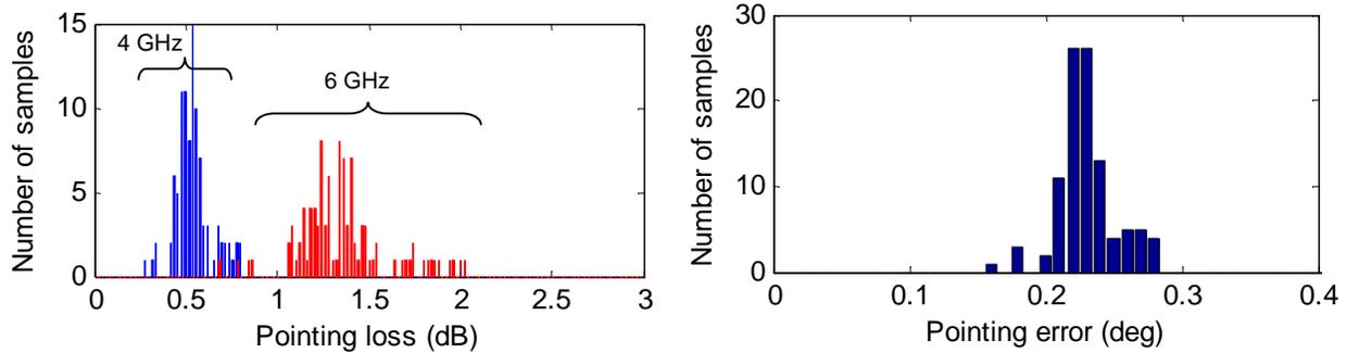
Figure 17. Pointing statistics using simple peaking.
