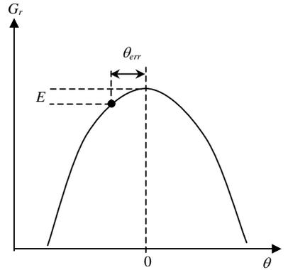
Figure 7. Simple peak pointing method.
