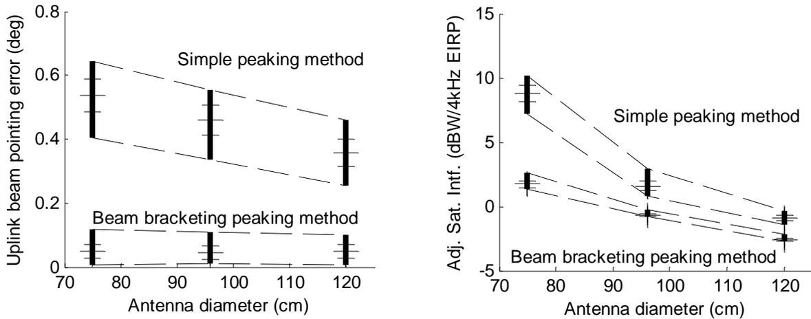
Figure 16. Ku VSAT pointing error and adjacent satellite interference levels.
