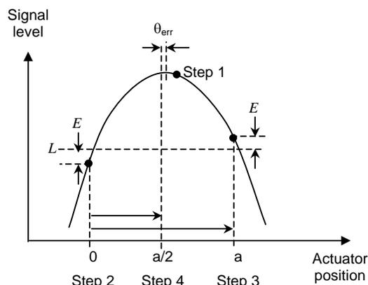
Figure 8. Beam bracketing pointing method.
