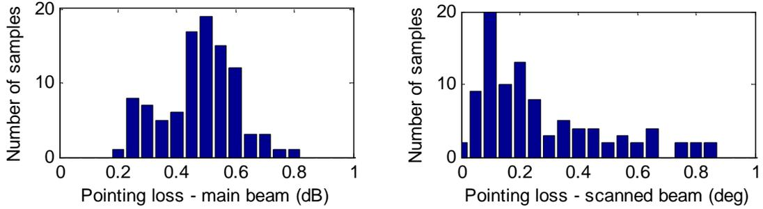
**Figure 12. Pointing statistics using simple peaking.**
