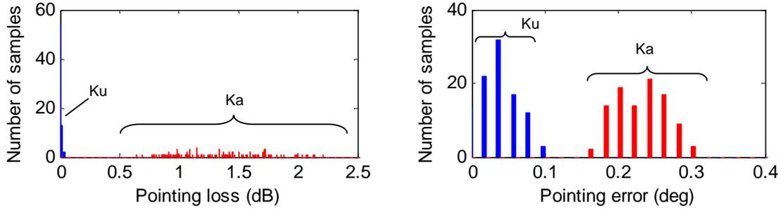
Figure 15. Pointing statistics using beam bracket peaking.
