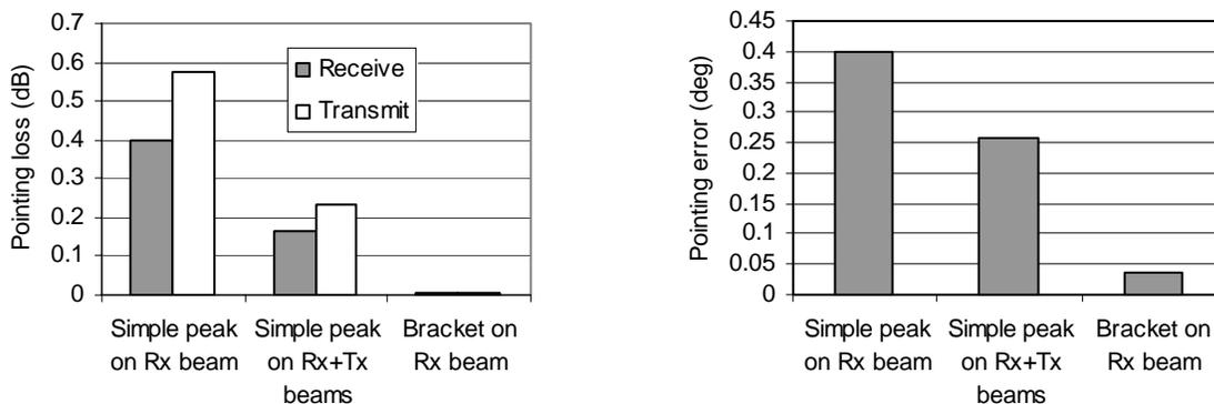
Figure 9. Comparison of pointing methods for a 0.75m Ku-band antenna.
