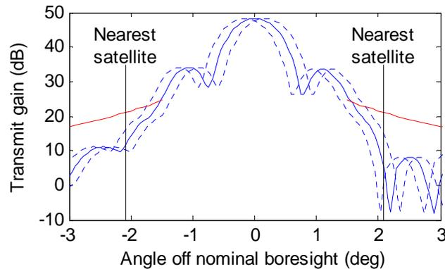
Figure 19. Andrew 4.9m antenna, transmit beam.
