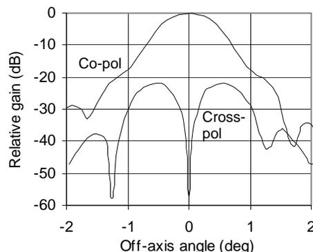
Figure 10. Example offset reflector antenna patterns.
