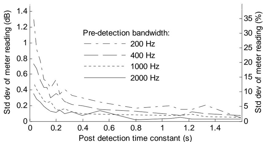
Figure 5. Standard deviation of signal meters measuring noise-like signals.
